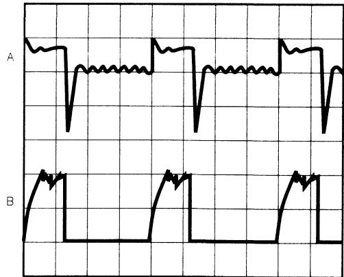
Figure 2. Switching on in Discrete Increments (trace A), Fig 1's Driver IC Forces Current (traces B) into the Motor to Speed it up. Upon Reaching Equilibrium, the Circuit Oscillates Around the Setpoint
